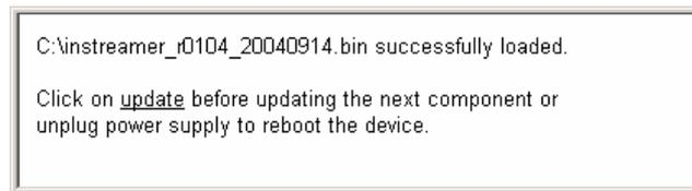
Click on the update link before updating the next component. Unplug power supply to reboot the device or type "reboot" in the resource field (without the ")
