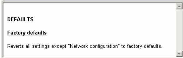
Click on "Factory defaults" to revert all settings except "Network configuration" to factory defaults. While restarting the device the following screen appears showing a number counting down:
